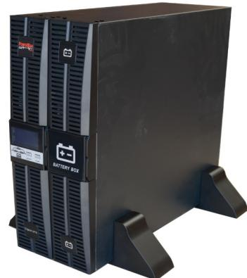
The UPS has a built in Static By-Pass feature which enables the machine to transfer the load to normal mains under certain emergency conditions, such as an overload. Once the condition causing the by-pass has been corrected the unit will automatically return to its normal operating mode.
